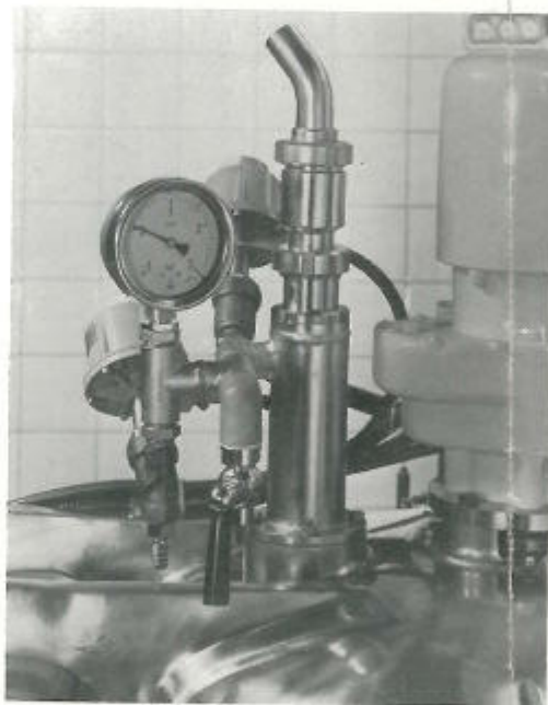
Pneumatically operated vacuum and ventilation valve, relief valve and manovacuummeter.
