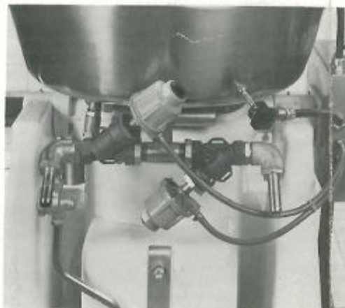
Connections for steam and water with pneumatically operated valves. Sensor for electronic temperature measurement.
