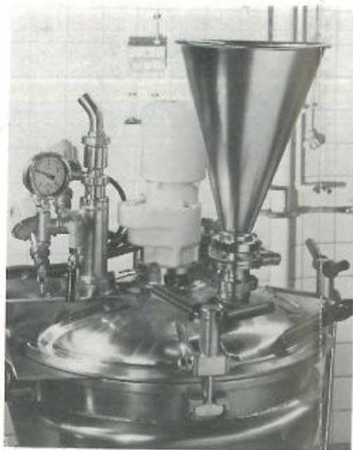
Dosing funnel with level gauge and pneumatically operated slide valve on dosing aperture NW 65. With union and union nut.
