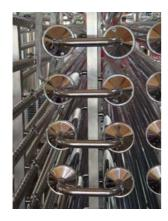
The ViscoLines can be manufactured with different surface finish and can be electropolished if required
