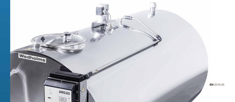
The manhole has a flexible lid that seals without rubber seal. A rubber seal is available on request.
